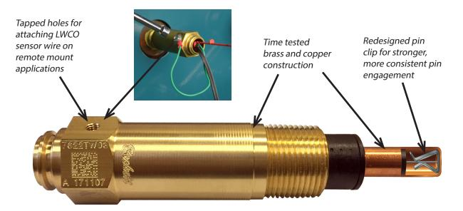
Machined brass bodies for strength and consistent threads
