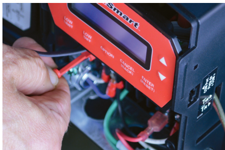
Figure 12 – Inserting Sensor in Well
