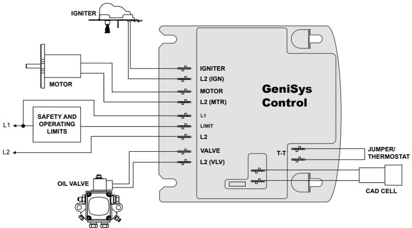
**NOTE:** Motor-off delay on a 7580P will be disabled if the safety and operating limits, shown in this figure, interrupt power to the control terminal L1. Connect thermostat leads to the TR and TW terminals on the control or jumper the TR and TW terminals on the control as directed by the appliance wiring diagram.
