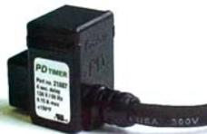
The PD Timer delay cordset is a direct replacement for standard oil burner solenoid valve cordsets but contains electronics that provide a precise 4 sec. delay before the valve coil is energized. It is designed to plug into 120 VAC solenoid valves such as the Beckett / Delta F84 valve and the **CLEANCUT** and Suntec valves, to provide a valve-on delay with primary controls that do not provide the delay.
