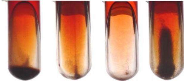
These test tubes contain untreated fuel that was “aged” four months by a heating process. The samples, which were among many collected from around the county, show the variability in fuel stability.
