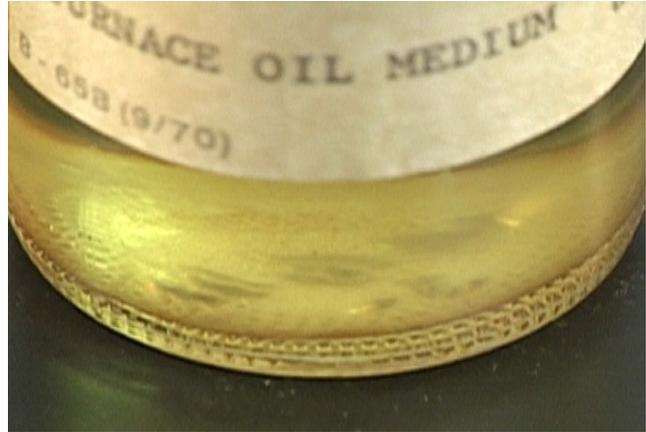
**Prior to the 1970's, most heating oil was produced by a simple distillation process. This fuel sample is almost 35 years old and has produced virtually no sediment.**
