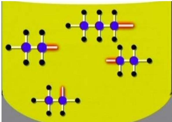
Active ends (shown in red) of artificially cracked hydrocarbon chains are the source of instability in today’s fuels. Over time, these ends recombine, forming long chain molecules (heavy oils) in stored fuel.
