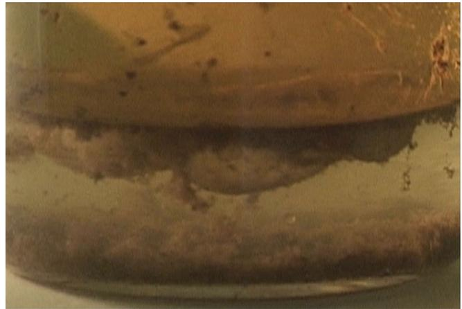
Bacterial, fungal or algae growth can occur in stored heating oil. However, service problems due to microbial contaminants are much less common than are those resulting from repolymerized fuels.
