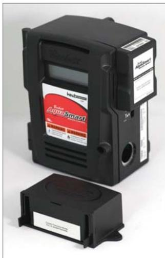
The Beckett AquaSmart® Wireless Temperature Module (WTM) is a 2-part accessory for the AquaSmart boiler control. It adds outdoor reset capability to the AquaSmart control by overriding the control's built-in HeatManager algorithm when installed. The wireless feature makes installation easy by eliminating mounting location limitations for the outdoor sensor and the need to run wires outside. Outdoor Temperature Reset
