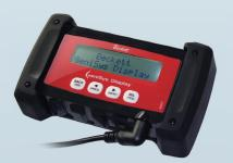
The GeniSys® Contractor Tool (Pt. No. 52082U) allows a technician to monitor and program the primary control variables. The display shows current burner status, control timings, and burner cycle history. The display's programming mode allows a technician to customize both the pretime and post-time settings and a lockout service message.
